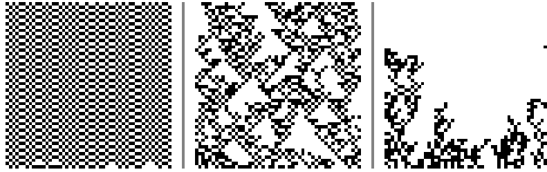
Figure 11: Simulation of the evolution of the \alpha -dependent elementary cellular automata 50: (left) \alpha = 1.0 (centre) \alpha = 0.75 (right) \alpha = 0.5 . The critical value of \alpha for this automaton is approximatively \alpha_c = 0.63 .
